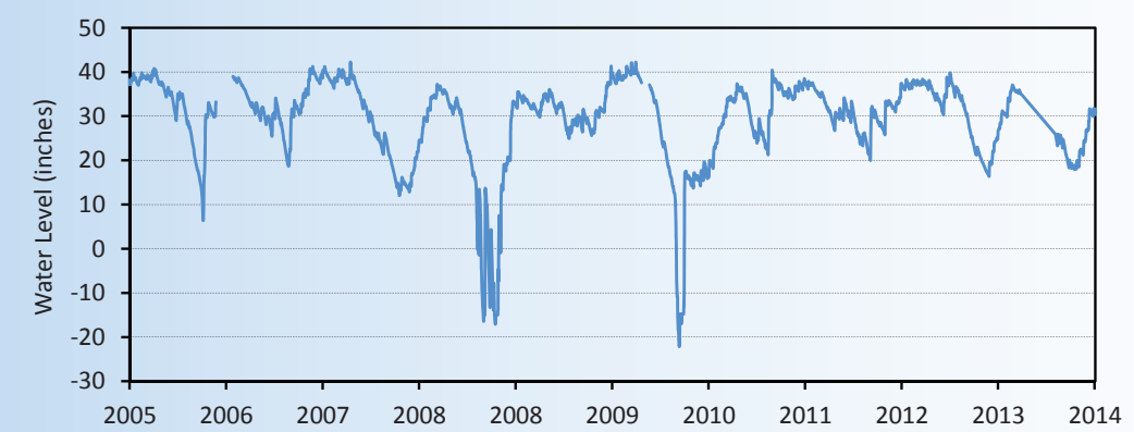
A water-level graph for a Pinelands pond. Zero represents the ground, values above zero indicate surface-water depth in the pond, and values below zero show the groundwater level after the pond dries.
